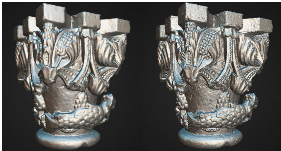
Figure 3: the model on the left shows the mesh without the normal map applied, the model on the right shows the mesh with normal map applied. Model: "Capitell de les Sirenes", Museums of Sant Cugat. Programa Giravolt. Author: Pol Guiu Alargé (La Tempesta). Reference: https://skfb.ly/oEJLo
